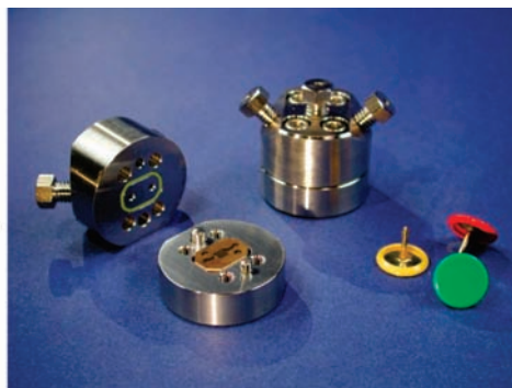
Figure 1. Mixing principle and setup of the slit-interdigital mixer. The inner volume of the micromixer is 8 \mu\text{L} . Mixing takes place by very fast diffusion between the thin reactant layers formed by the parallel microchannel alignment.
